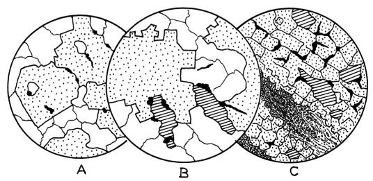
Fig.3. Drawings of polished sections of Bimbimbie ore. Gold shown in black; pyrite dotted; chalcopyrite lined and quartz unshaded. Magnified x35.
