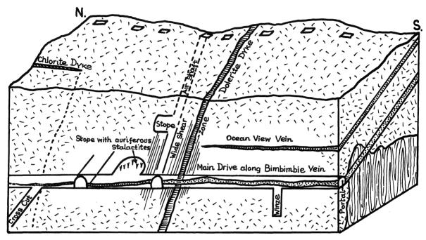
Fig.2. Bimbimbie gold mine showing relevant geology and underground workings. Centre left is stope containing limonitic stalactites. Length of section about 500 m. The section oriented North-South in order to show greater detail.
