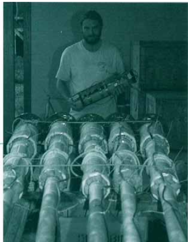
Jason Gedamke loads batteries into hydrophones in the Purves Laboratory for deployment off Lizard Island to track minke whales.
